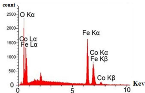
Fig. 5: EDX analysis of porous nanoparticle.
