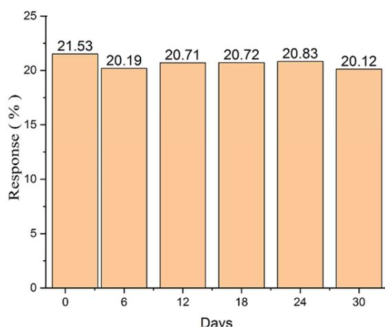
Fig. 12: Response of sensor to 100 ppm methanol vapors in 30 days.
