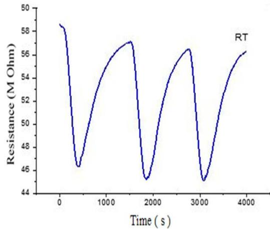
Fig. 11: Repeatability of sensor to 100ppm methanol vapors at room temperature.
