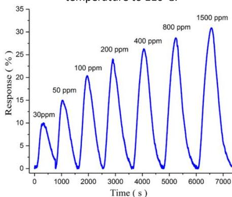
Fig. 7: Response of sensor in different methanol vapors concentrations (30ppm to 1500 ppm).
