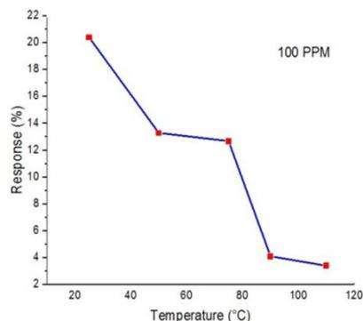
Fig. 6: Response of methanol sensor to different temperature for 100ppm methanol vapors in room temperature to 110°C.
