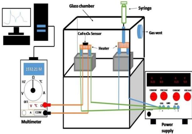
Fig. 2: The setup for measuring sensor's resistance before and after exposing the methanol vapors.
