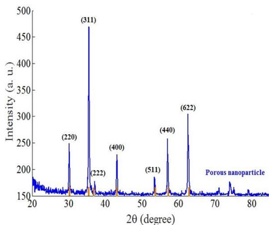
Fig. 3: XRD pattern of porous nanoparticles.
