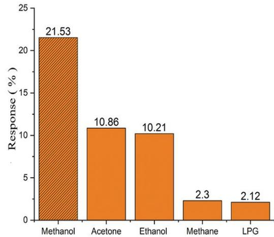
Fig. 10: Response of sensor to 100ppm methanol, acetone, ethanol, methane and LPG at room temperature.
