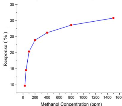
Fig. 8: Response of sensor in different methanol concentrations in 30 ppm to 1500 ppm at room temperature.
