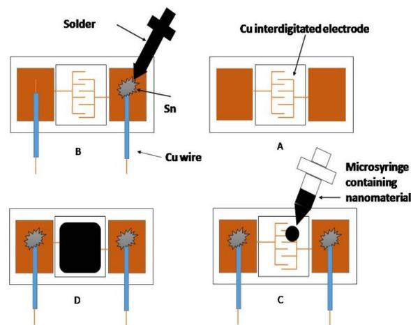
Fig. 1: The process of sensor fabrication, (A) A schematic picture to show the substrate, (B) Connecting Cu wires to PCB substrate by solder, (C) Adding 0.05 ml of ferrite cobalt porous nanoparticles in Cu interdigitated electrodes by micro syringe, (D) The prepared sensor.
