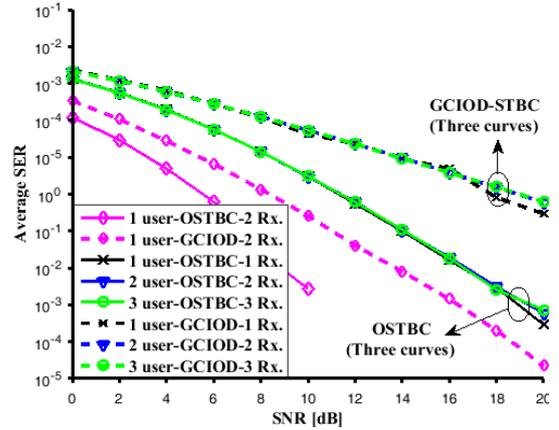
Fig. 2: SER comparison of receiver for transmissions of OSTBC and GCIOD-STBC schemes over different scenarios having  $N = 2$  transmitting antennas.
