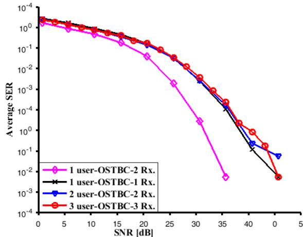
Fig. 5: SER comparison of receiver for transmissions of Alamouti design using 16-QAM constellation.
