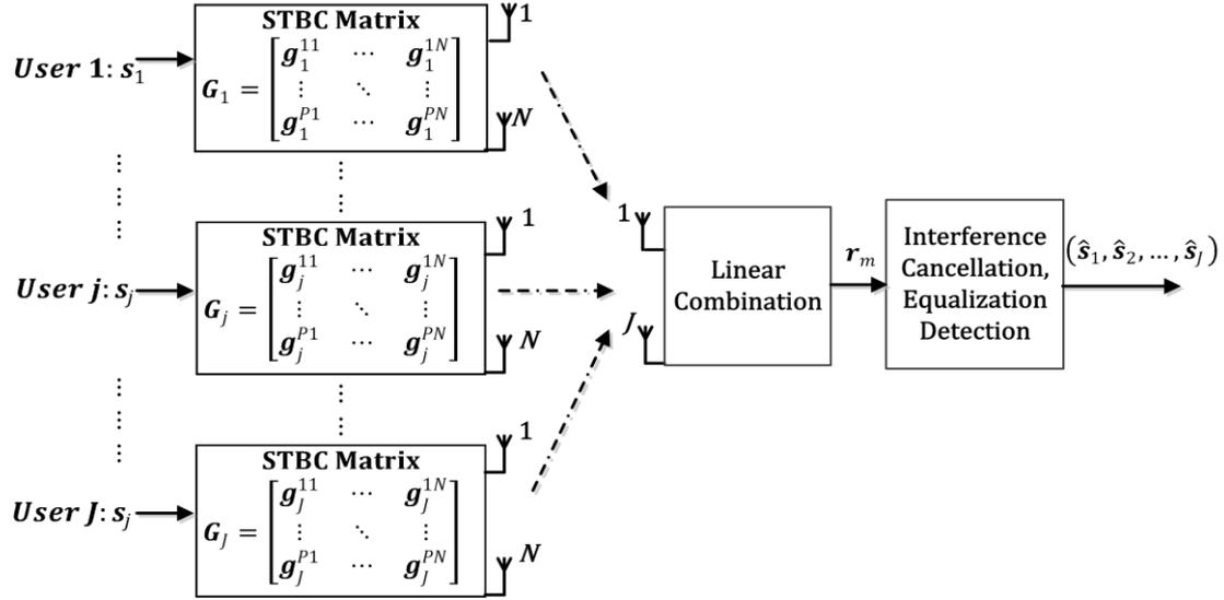
Fig. 1: Transceiver block diagram for a MIMO multiple-access system.
