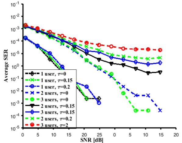
Fig. 6: SER comparison of receiver for transmissions of Alamouti design in the presence of channel estimation error.
