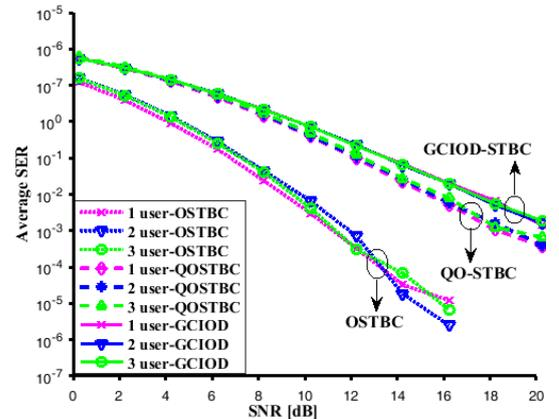
Fig. 3: SER comparison of receiver for transmissions of OSTBC, QO-STBC and GCIOD-STBC schemes over different scenarios having  $N = 4$  transmitting antennas.
