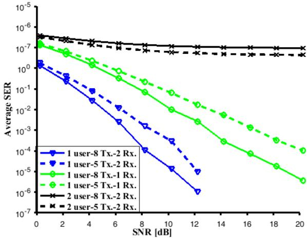
Fig. 4: SER comparison of receiver for transmission of half-rate OSTBC designs having  $N=5$  and  $N=8$  transmitting antennas.
