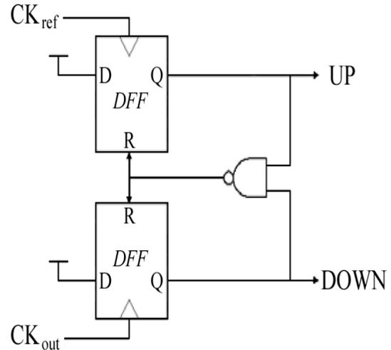
Figure 4: Flip-flop based PFD
