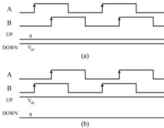
Figure 6: Different states of designed PD, (a) Signal A is the leading signal, (b) Signal B is the leading signal
