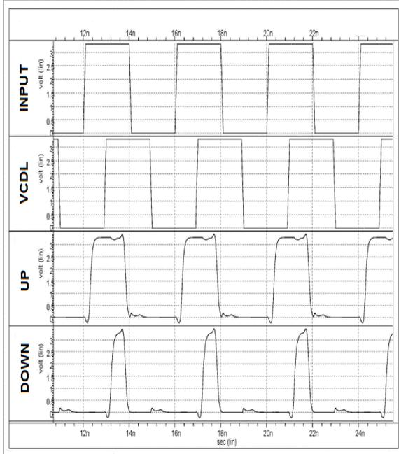
Figure 13: Simulation results for flip-flop based PFD
