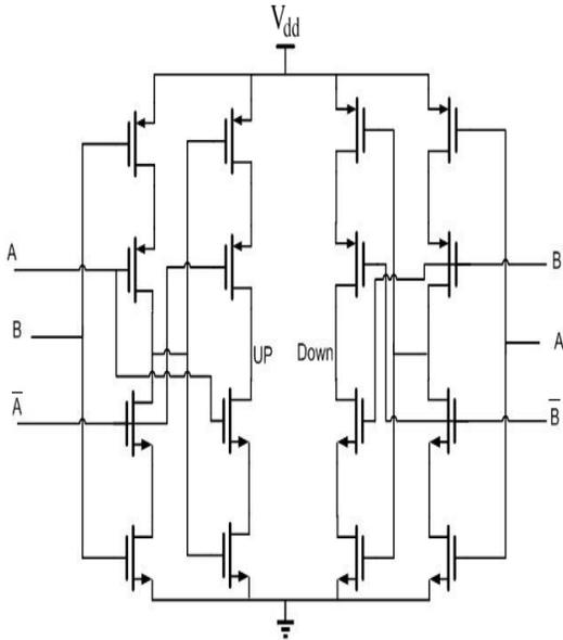
Figure 5: Designed PD circuit
