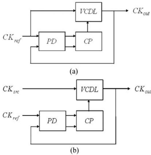
Figure1: Common architectures of DLL (a) For signal synchronization purposes (b) For clock recovery purposes
