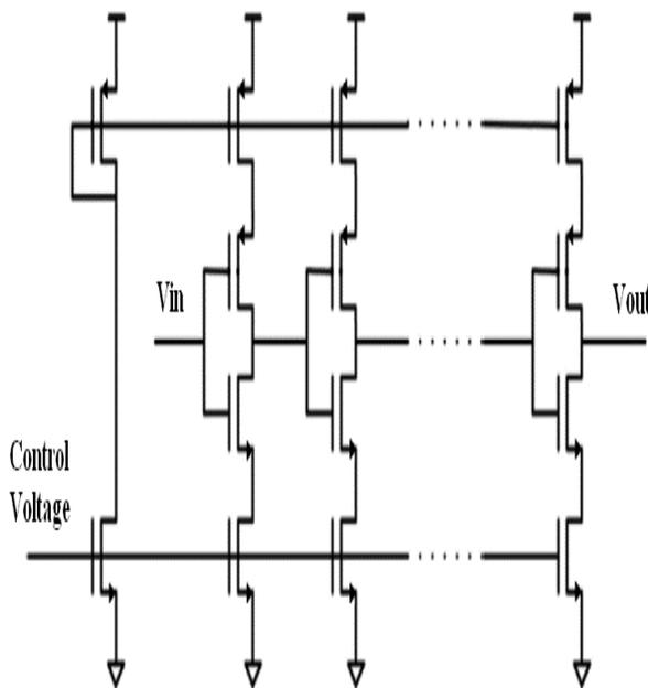
Figure 11: Inverter based VCDL
