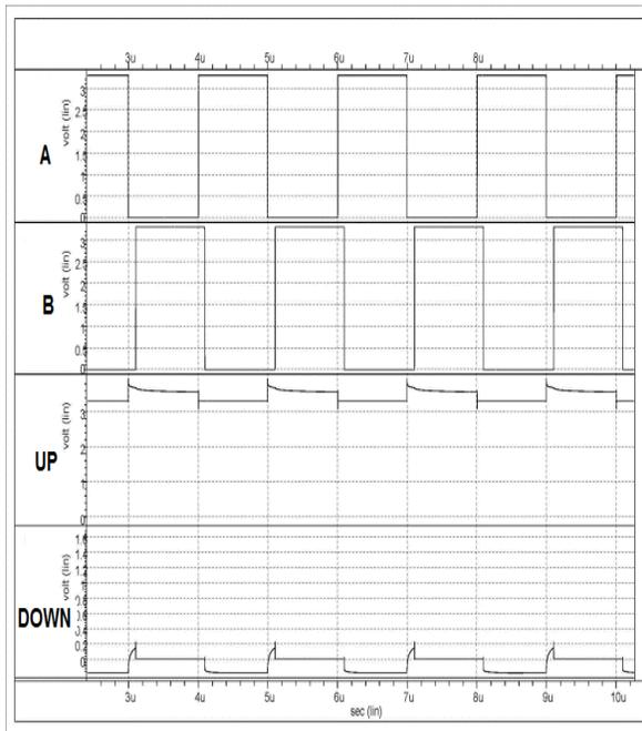
Figure 14: Simulation results of proposed PD
