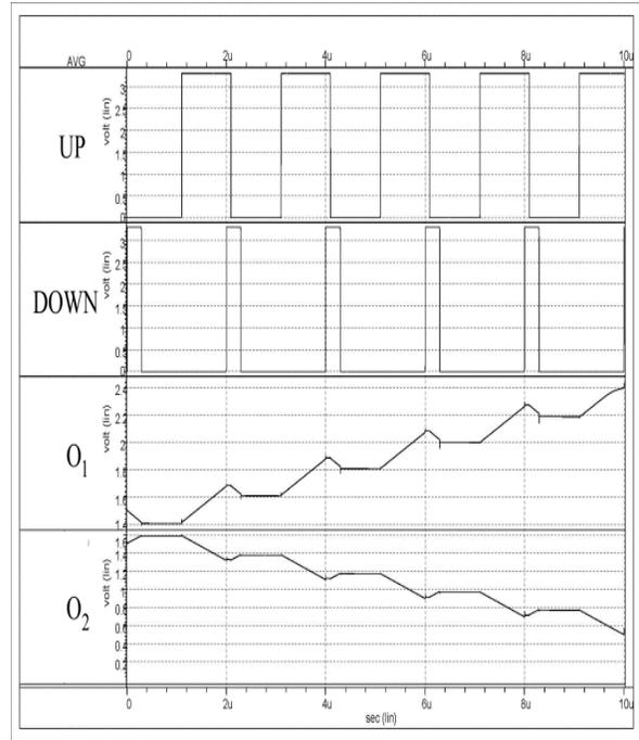
Figure 15: Simulation results of proposed CP.
