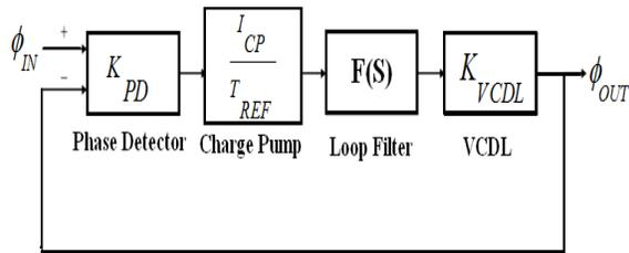
Figure2: S-domain model of a DLL in terms of phase
