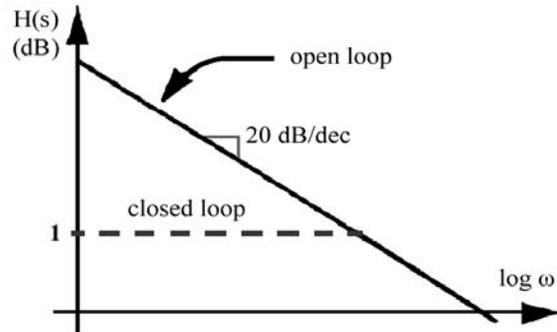
Figure3: First-order transfer function of a DLL
