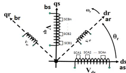
Fig. 2: The schematic of the resolver's windings.
