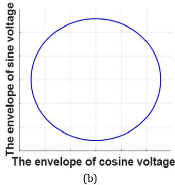
Fig. 5: The results of the healthy sensor obtained from the proposed model: (a) Analogue voltages, (b) The envelope of sine voltage versus that of cosine voltage.
