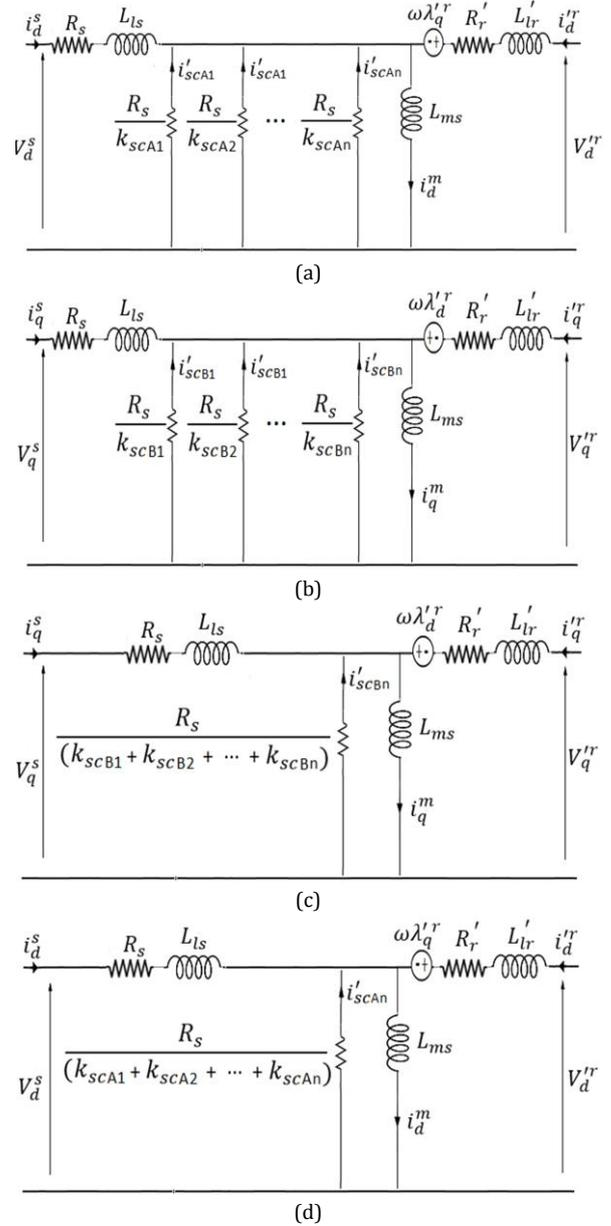
Fig. 3: The equivalent circuit of the studied WR resolver under short circuit fault: (a) d-axis equivalent circuit, (b) q-axis equivalent circuit, (c) Simplified equivalent circuit of d-axis, and (d) Simplified equivalent circuit of q-axis.
