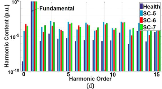
Fig. 6: The harmonic content of the voltages' envelope: (a) for the sine voltage (independent faults), (b) for the cosine voltage (independent faults), (c) for the sine voltage (simultaneous faults), and (d) for the cosine voltage (simultaneous faults).
