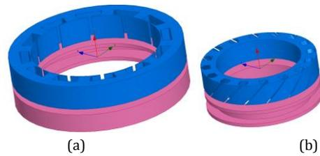
Fig. 1: The schematic of the studied brushless resolver: (a) The stator and the primary of RT, (b) The rotor and the secondary of RT.
