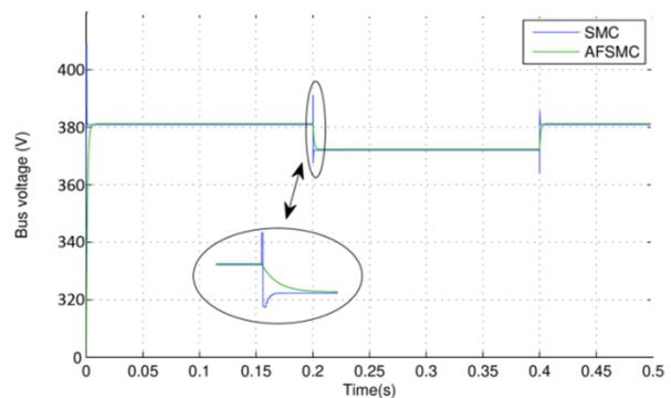
Fig. 10: The microgrid bus voltage.
