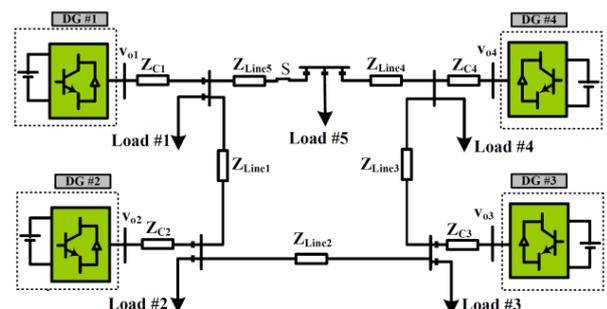
Fig. 11: An islanded four-DG microgrid test system.
