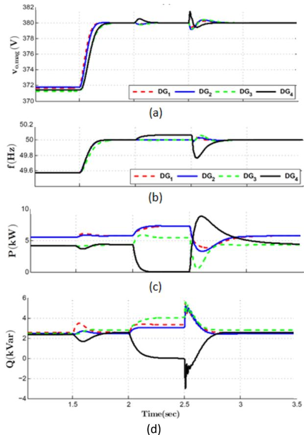
Fig. 13: The response of the microgrid to the disconnecting and reconnecting of DG#4, (a) terminal voltage of DGs; (b) Frequency of DGs; (c) Active power of DGs; (d) Reactive power DGs.
