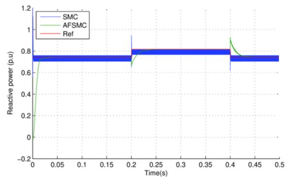
Fig. 9: Generator output reactive power.
