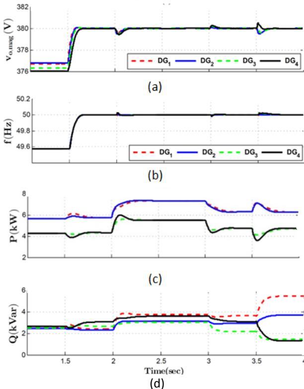
Fig. 12: The response of the microgrid to a multiple fault, (a) terminal voltage of DGs; (b) Frequency of DGs; (c) Active power of DGs; (d) Reactive power DGs
