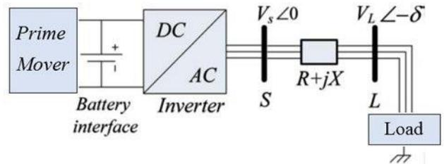
Fig. 1: A simple microgrid with inverter.
