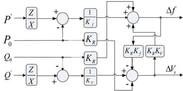
Fig. 2: The GDC block diagram of voltage and frequency control.
