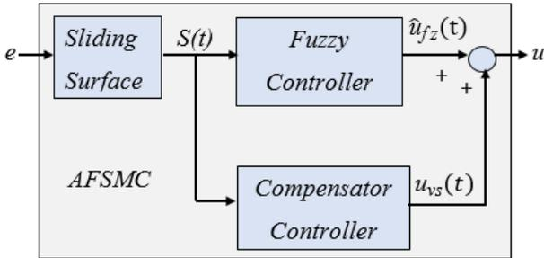
Fig. 4: Suggested controller block diagram.
