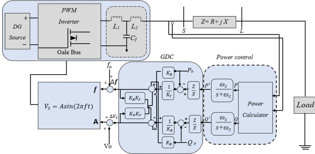
Fig. 3: Microgrid with conventional block diagram for VSI.
