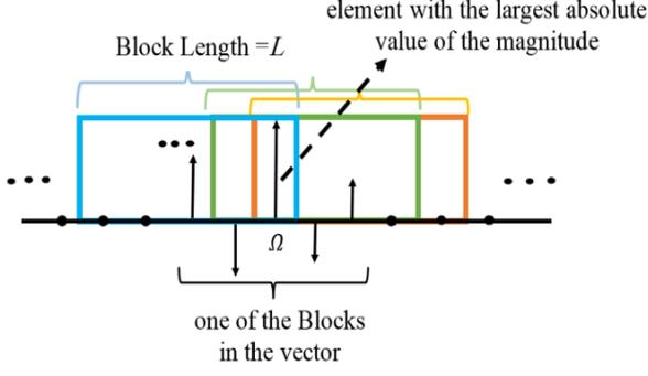
Fig. 2: Method of the finding a block in the block-sparse vector via the proposed algorithm.
