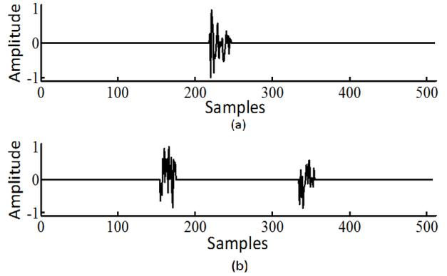
Fig. 3: Two types of measured acoustic-echo-channels as the unknown block-sparse systems, (a) one cluster, (b) two clusters.
