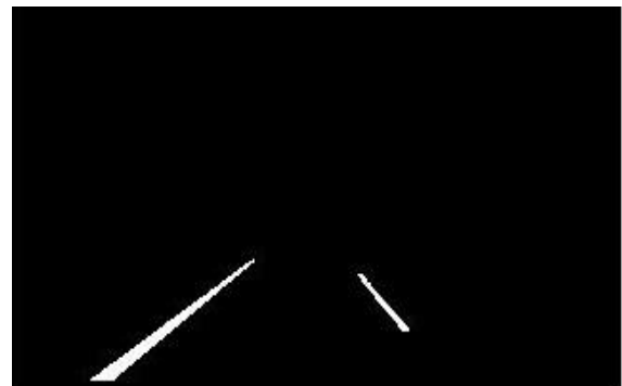
Fig. 7: Binary image after applying a mask.
