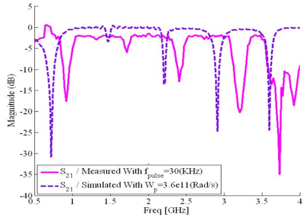
Fig. 14: The degree of conformity of the S<sub>21</sub> parameter in both simulated and measured modes.
