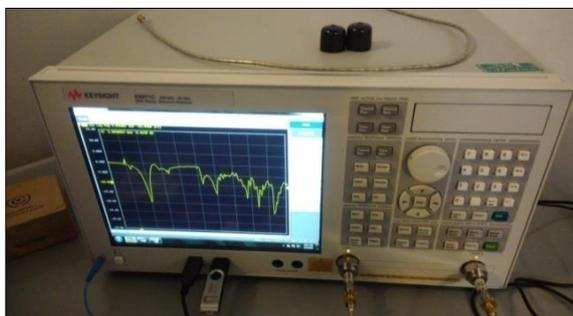
Fig. 10: Example of  $S_{21}$  parameter measurement with VNA.
