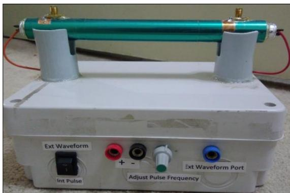
Fig. 6: Real view of plasma coaxial waveguide filter.
