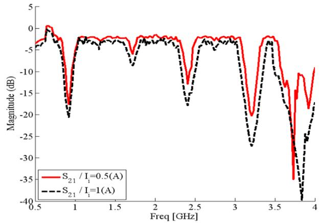
Fig. 13: S<sub>21</sub> Parameter measurement at 30 kHz with increasing plasma excitation input current.
