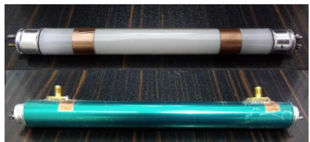
Fig. 8: Connecting the capacitive signal coupler to the fluorescent tube.
