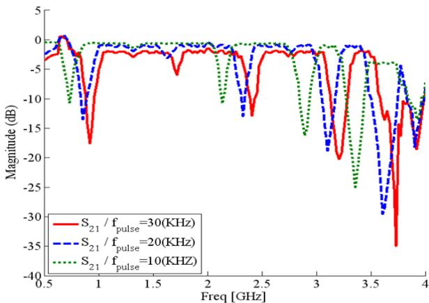
Fig. 12: S<sub>21</sub> Parameter measured with different excitation frequencies
