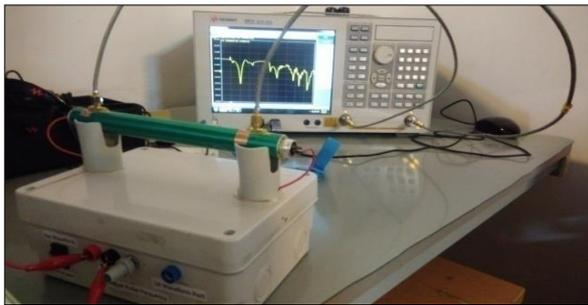
Fig. 9: Measurement of waveguide filter parameter with VNA.
