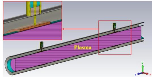
Fig. 1: Capacitive coupler view with connector and cut view of coaxial plasma waveguide filter.
