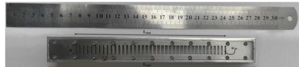
Fig. 8: The photograph of the fabricated antenna.
