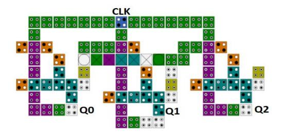
Fig. 13: The structure of proposed multilayer 3-bits counter.
