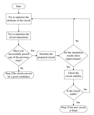
Fig. 10: The flowchart of the design methodology.
