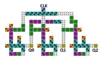
Fig. 1: Structure of three-bits counter with 110 cells [13].
