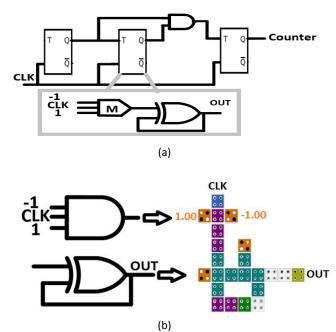
Fig. 11: (a) Block diagram of three bits counter. (b) Structure of 'AND' and 'XOR' gates.
