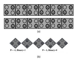
Fig. 9: (a) standard wiring. (b) complimentary chain wiring.
