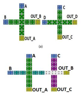
(b) Fig. 5: Coplanar wires (a) Two wires crossing in 45& 90degrees. (b) Two wires crossing with 2 different clock phases.
