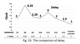
Table 1 shows all the parameters of the proposed design and the previous studies. The work in [13] has better parameters compared to the others, and therefore, our circuit has been compared to it. As seen, the delay has improved by 33.33%. The cells number decrement is 12.72% and the area reduction is 27.27%. A QCA specific cost function estimation is proposed in [24] that takes into account the number of logic gates and crossings wires in cost evaluation.
