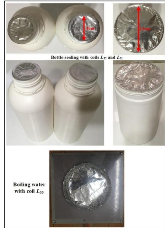
Fig. 14: Examples of sealed bottles with the coils L_{32} and L_{31} and boiling water with coil L_{33} .
