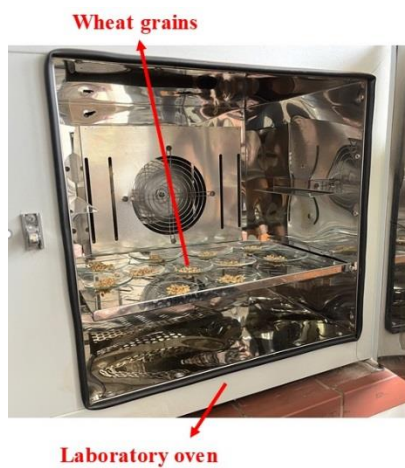
Fig. 7: Experimental setup for MC determination according to the ASAE S352 standard.
