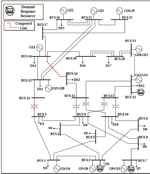
Figure 3: Single line diagram of RTS with DRRs.
