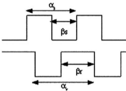
Figure 5: Pole pitch,  $\alpha_s$  and  $\alpha_r$ , and pole width,  $\beta_s$  and  $\beta_r$ , for both stator and rotor.
