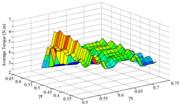
Figure 6: The changes of average torque in the range of  $0.53 \leq \gamma_s \leq 0.73$  and  $0.33 \leq \gamma_r \leq 0.53$ .
