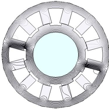
Figure 4: Contour plot of magnetic flux obtained by finite element analysis.
