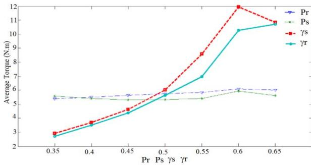
Figure 2: The changes of the average torque versus design parameters, including  $P_s, P_r, \gamma_s$  and  $\gamma_r$ .
