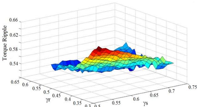
Figure 7: The changes of the torque ripple in the range of  $0.53 \leq \gamma_s \leq 0.73$  and  $0.33 \leq \gamma_r \leq 0.53$ .
