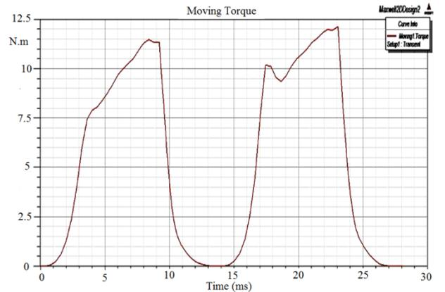
Figure 1: A typical waveform of the moving torque produced by SRM.
