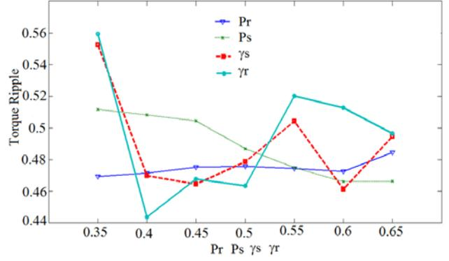
Figure 3: The changes of the torque ripple versus design parameters, including  $P_s, P_r, \gamma_s$  and  $\gamma_r$ .
