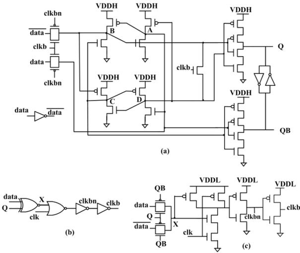
Figure 6: (a) The proposed LP-HRFF, (b) low supply voltage pulse generator circuit in logical level and; (c) in transistor level.
