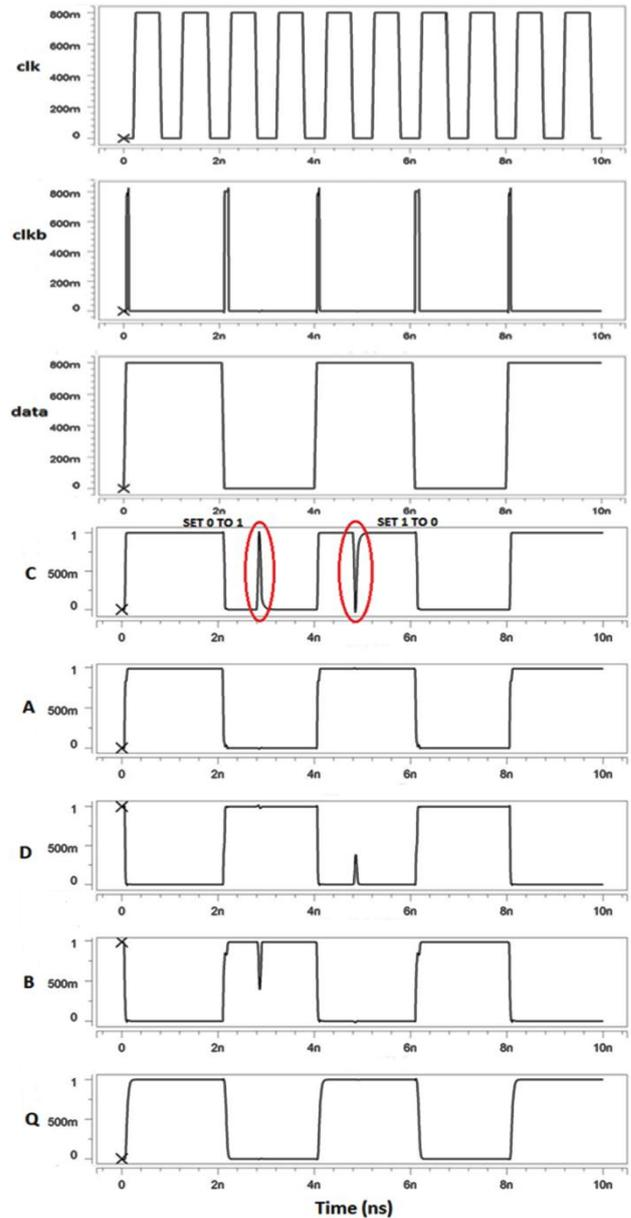
Figure 8: Waveforms of the proposed flip flop and SEU injection at node C.
