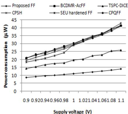
Figure 11: Power consumption versus different supply voltages.
