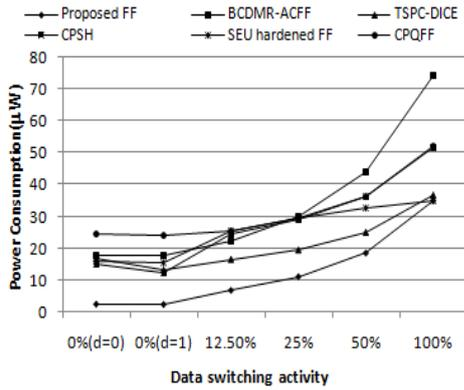
Figure 10: Power consumption versus different data switching activities.
