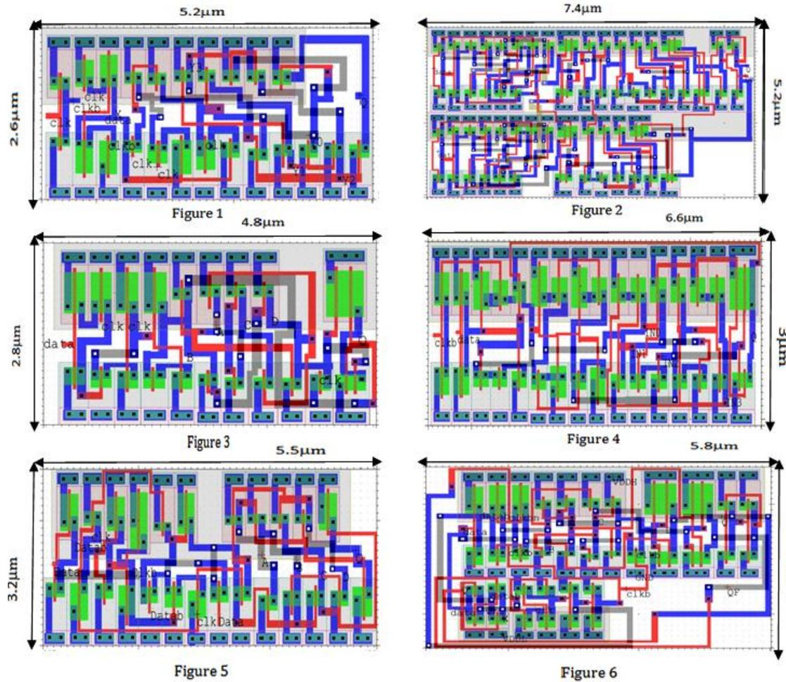
Figure 18: Flip-Flops layouts in CMOS technology.
