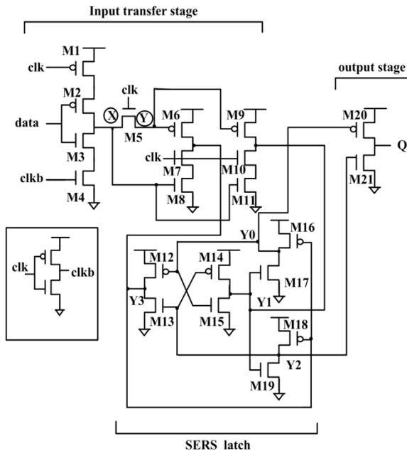
Figure 1: CPSH flip-flop [10].
