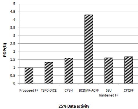
Figure 9: The comparison of power delay product for 25% data switching activity.
