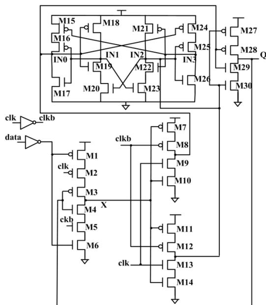
Figure 4: SEU hardened flip-flop [5].
