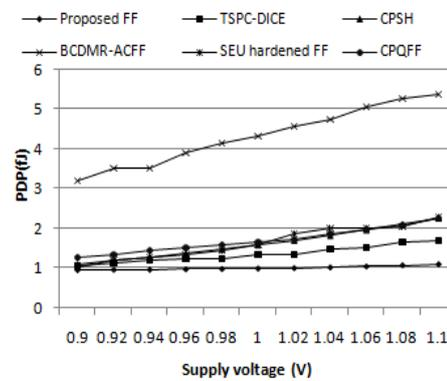
Figure 13: PDP versus different supply voltages.
