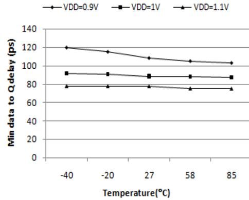
Figure 12: Minimum data-to-Q delay versus temperature in different voltages.
