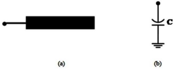
Fig. 3: (a) Open-end, (b) Equivalent LC circuit.
