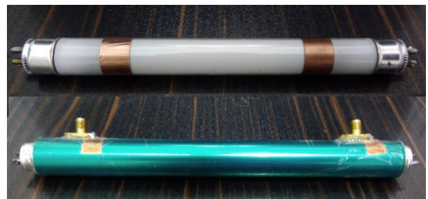
Fig. 8: Connecting the capacitive signal coupler to the fluorescent tube.
