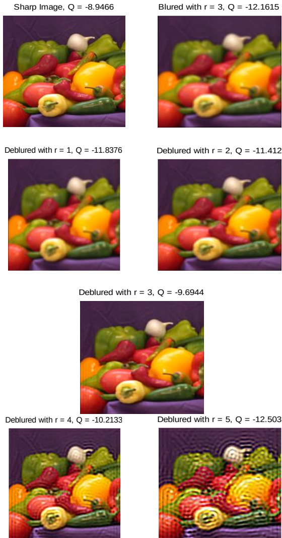
Fig. 7: Deblurring results with different radii of the kernel ( r=1..5 ) in imaging with conventional aperture. Deblurring with smaller kernels results in blurry images and deblurring with larger PSFs yields images with artifacts. The quality of each image is evaluated by the no-reference quality assessment measure proposed in [36]. A larger Q-value indicates higher quality.
